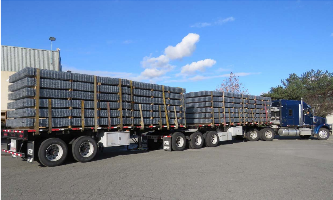
Load of welded wire reinforcement mesh
