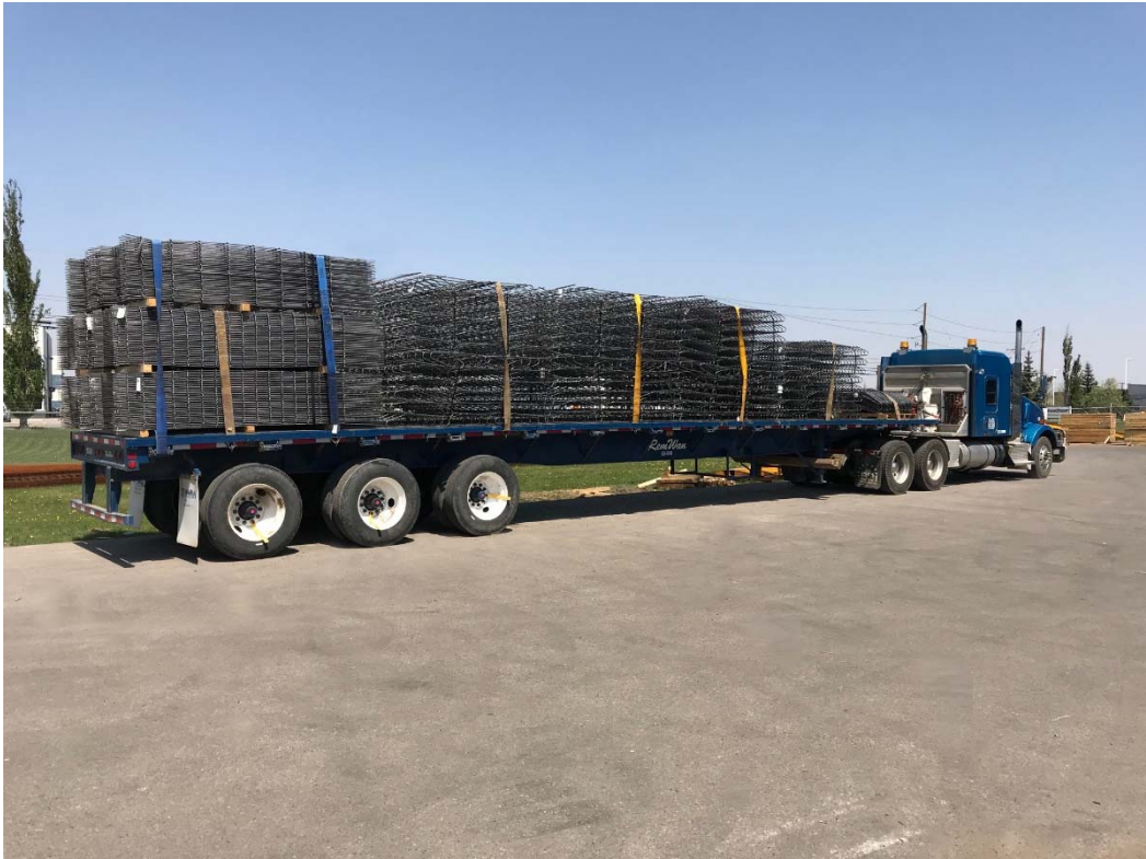
Shipment of Engineered Structural Mesh in Calgary used for concrete reinforced girders on a bridge overpass.
